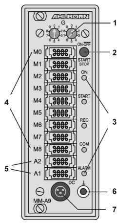
8690-9A only, recharg. battery pack AP : (8) Connection socket DC-A 12V
