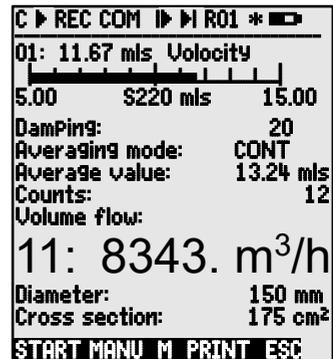
**Volume flow** VF = average flow velocity  $\bar{v}$  • cross section area CS:
