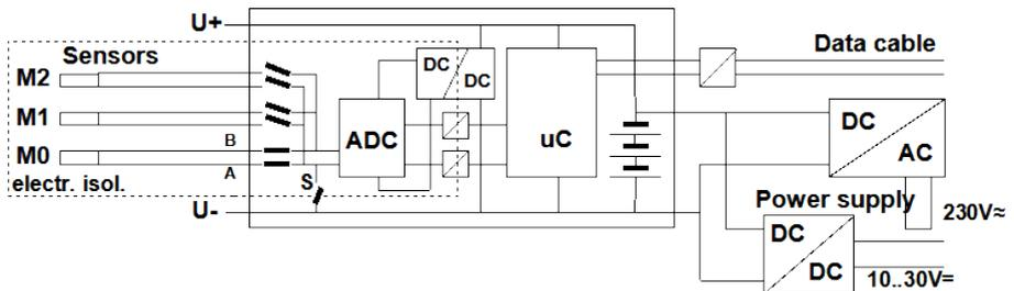
The 9 analog inputs are electrically isolated from each other by means of photovoltaic relays and - on this device for the first time - also from the device itself and from the power supply by means of optocouplers. Between all inputs and outputs (even the analog output cables which are not electrically isolated) the maximum potential difference permitted is 50 volts. The voltage at the measuring inputs themselves must not exceed 12 volts (between B, C, D, and A).
