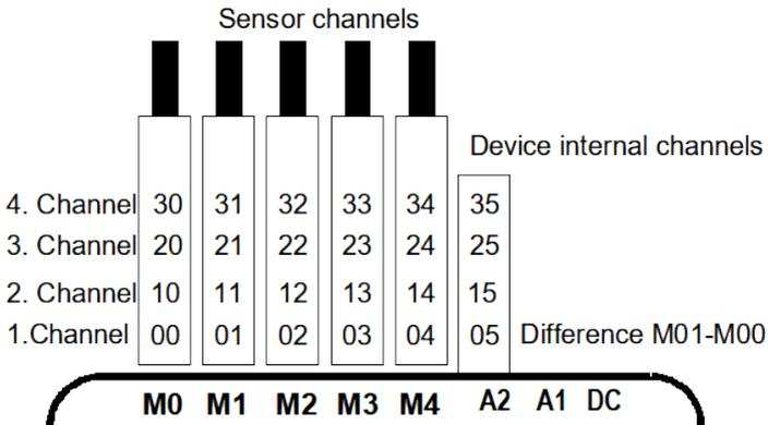
**A new feature is the presence of four device-internal channels:**
