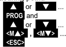
To **set the display range** for the bar chart the functions "**Analog start**" and "**Analog end**" in the "**Special functions**" menu should be used; (see 11.4.4). Having selected these functions they can be entered by pressing **PROG** and ▼ or directly on the appropriate axis; (see 9.5).
