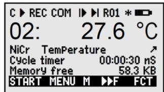
The device status is displayed by certain symbols in the status bar (see 9.2). Data acquisition can be set to cyclic via the **cycle timer**. The available memory is displayed in the function **memory capacity free**. This is omitted if neither internal memory nor a memory connector is available. The menu can then be used for output via the interface to a computer.
