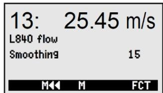
number of measured values to be averaged (possible range 0 to 99). The smoothed measured value can thus also be used in all subsequent evaluation functions in combination with averaging over individual measured values (see
